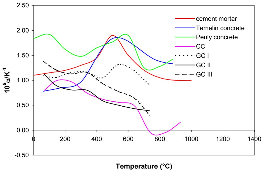
Fig. 2 Linear thermal expansion coefficient of cement based composites
