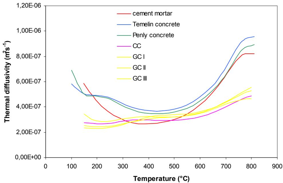
Fig. 1 Thermal diffusivity of cement based composites
