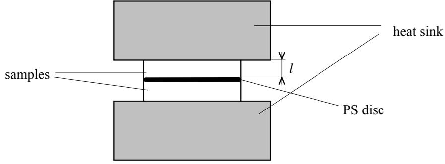
Figure 1. The setup of the experiment.
