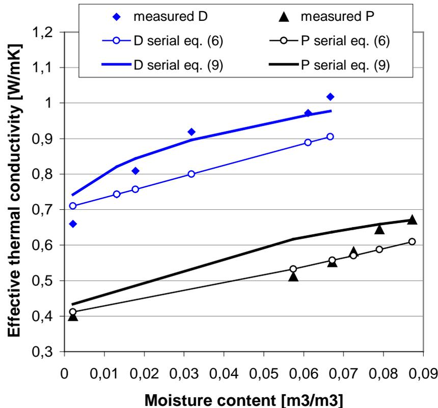
Fig. 3 Thermal conductivities of bricks D and P vs. moisture content. Comparison of the measured values and modeled values by eq. (6) and (9)
