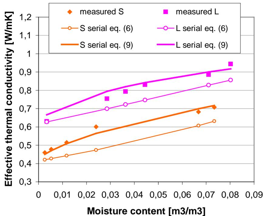
Fig. 4 Thermal conductivities of bricks S and L vs. moisture content. Comparison of the measured values and modeled values by eq. (6) and (9)
