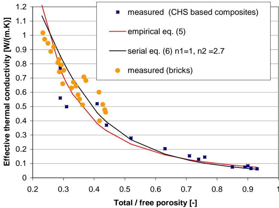
Fig. 1 Thermal conductivities of clay bricks and CHS based materials vs. total / free porosity. Comparison of the measured values with empirical approximation (5) and serial model (6)
