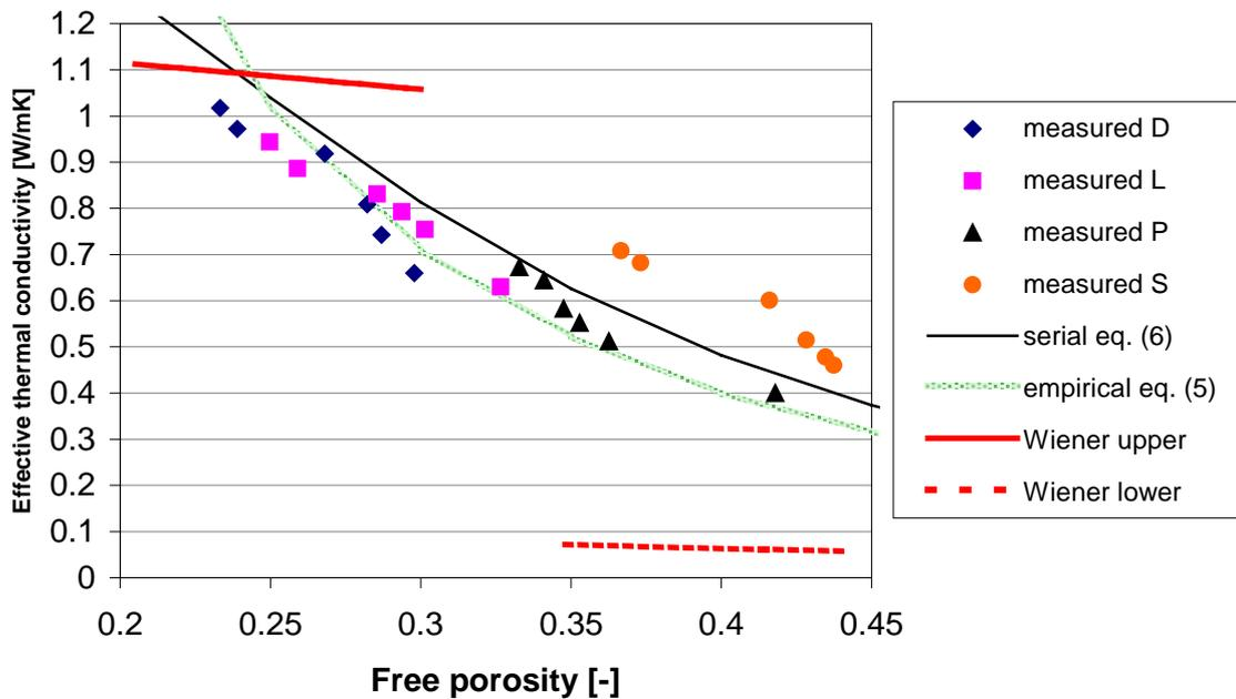
Fig. 2 Thermal conductivities of moist clay bricks vs. free porosity. Comparison of the measured values with empirical approximation (5), serial model (6) and Wiener bounds
