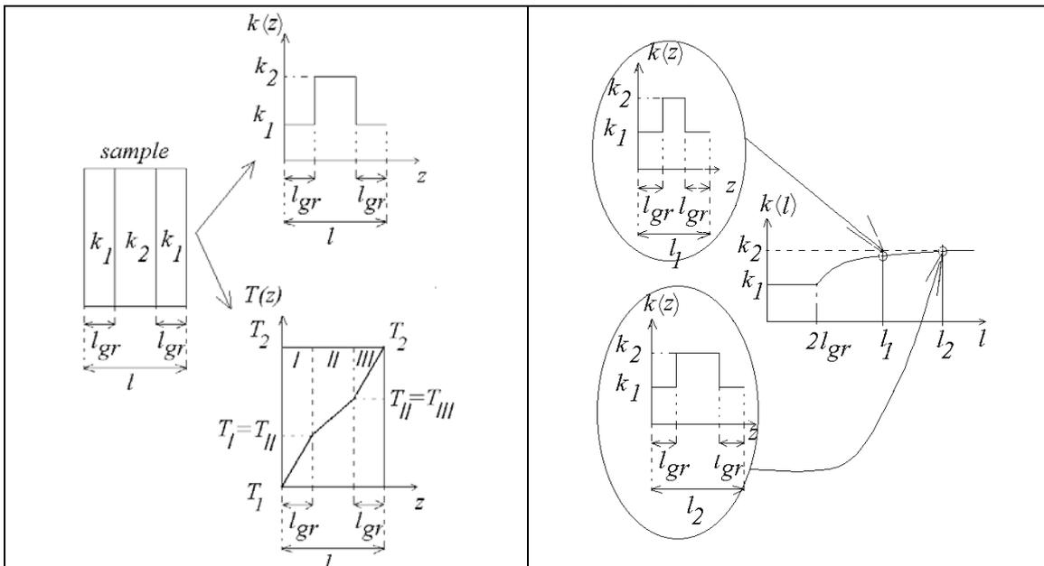
Fig. 3. The model of dependence of  $k(z)$  (for the sample thickness  $l$ ) accepted for analytical considerations [1]
