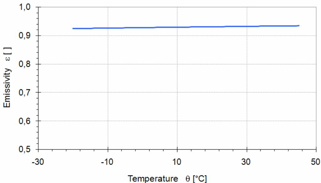
Figure 5: Overall emissivity  $\varepsilon$  of measured sample (the blue curve) depending on temperature. Calculated due to the equation (8), integrated numerically over the range of wavelengths for which spectral emissivity has been measured.
