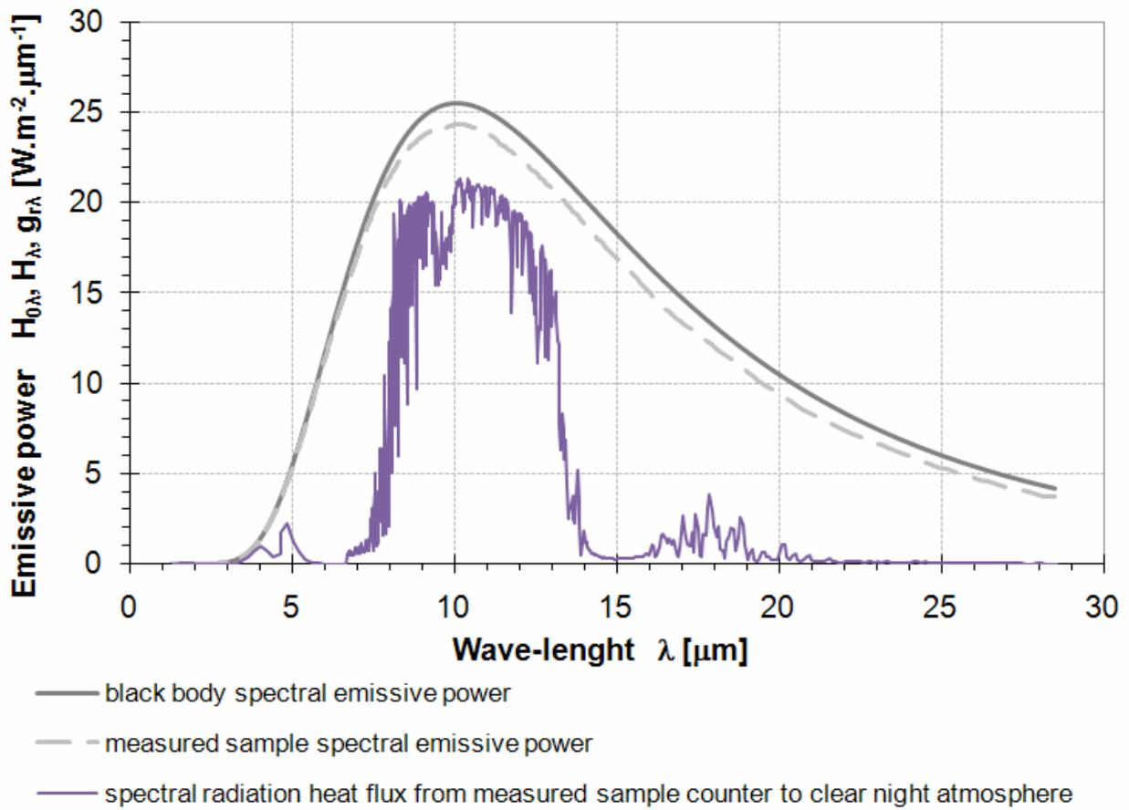
Figure 4: Calculated spectral radiation of black surface  $H_{\lambda 0}$ , in comparison with spectral radiation of surface  $H_{\lambda}$  of measured sample and spectral radiant heat flux  $q_{r\lambda}$  of sample surface oriented horizontally against clear night sky. All three curves of values of spectral surface radiation are calculated for temperature of radiating surface  $15^{\circ}\text{C}$ .
