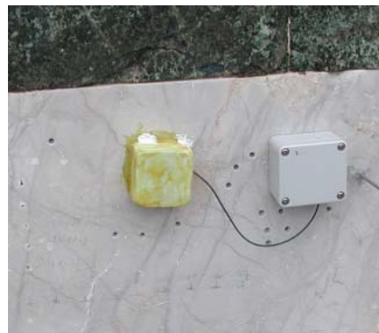
Fig.6.: Cupola of the Duomo Cathedral (left) and the fixing of the hot ball and the instrument RTM 1.01.
