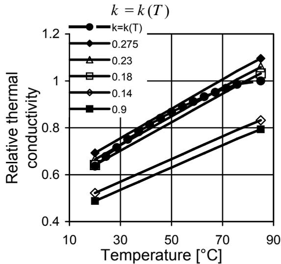
Figure 9. Thermal conductivity at various times of heating
