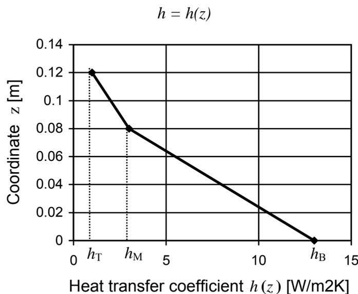
Figure 3. Changes of the heat transfer coefficient along the side surfaces of both cylinders
