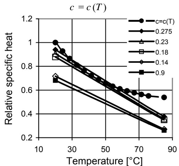
Figure 10. Specific heat determined at various times of heating
