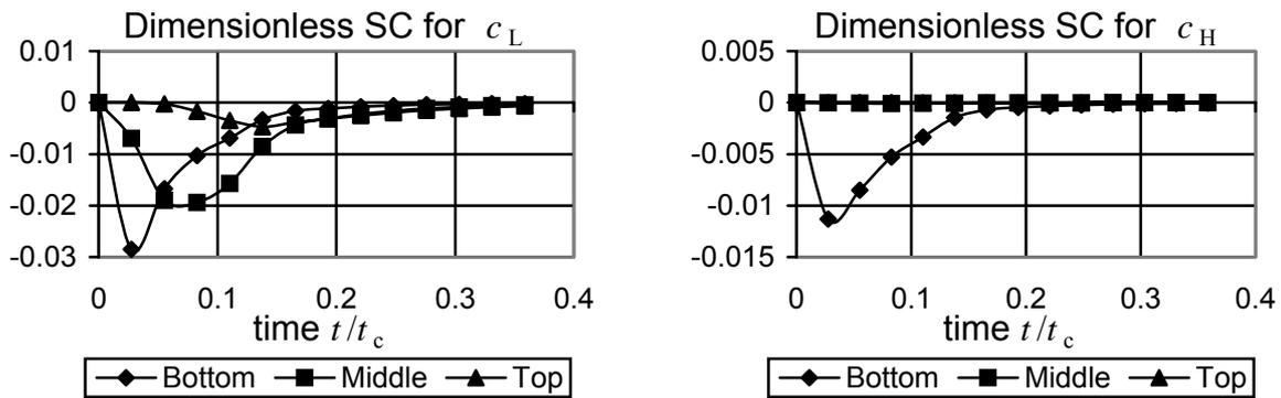
Figure 4. Dimensionless sensitivity coefficients for thermophysical parameters
