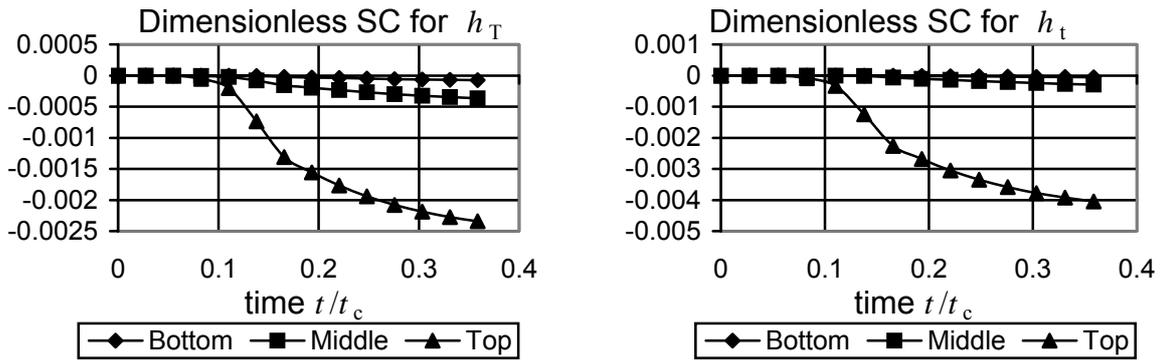
Figure 5. Dimensionless sensitivity coefficients for the boundary conditions
