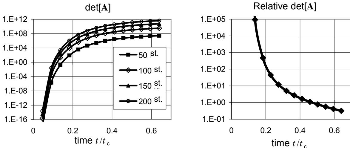
Figure 6. The determinant value changing with increasing time of heating and the different number of measurement point
