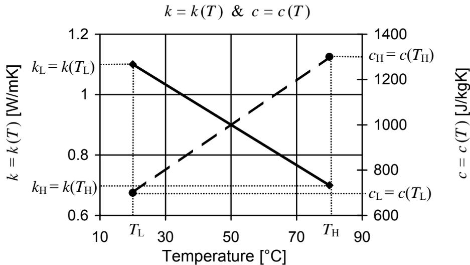
Figure 2. The temperature dependence of the thermal conductivity and the specific heat
