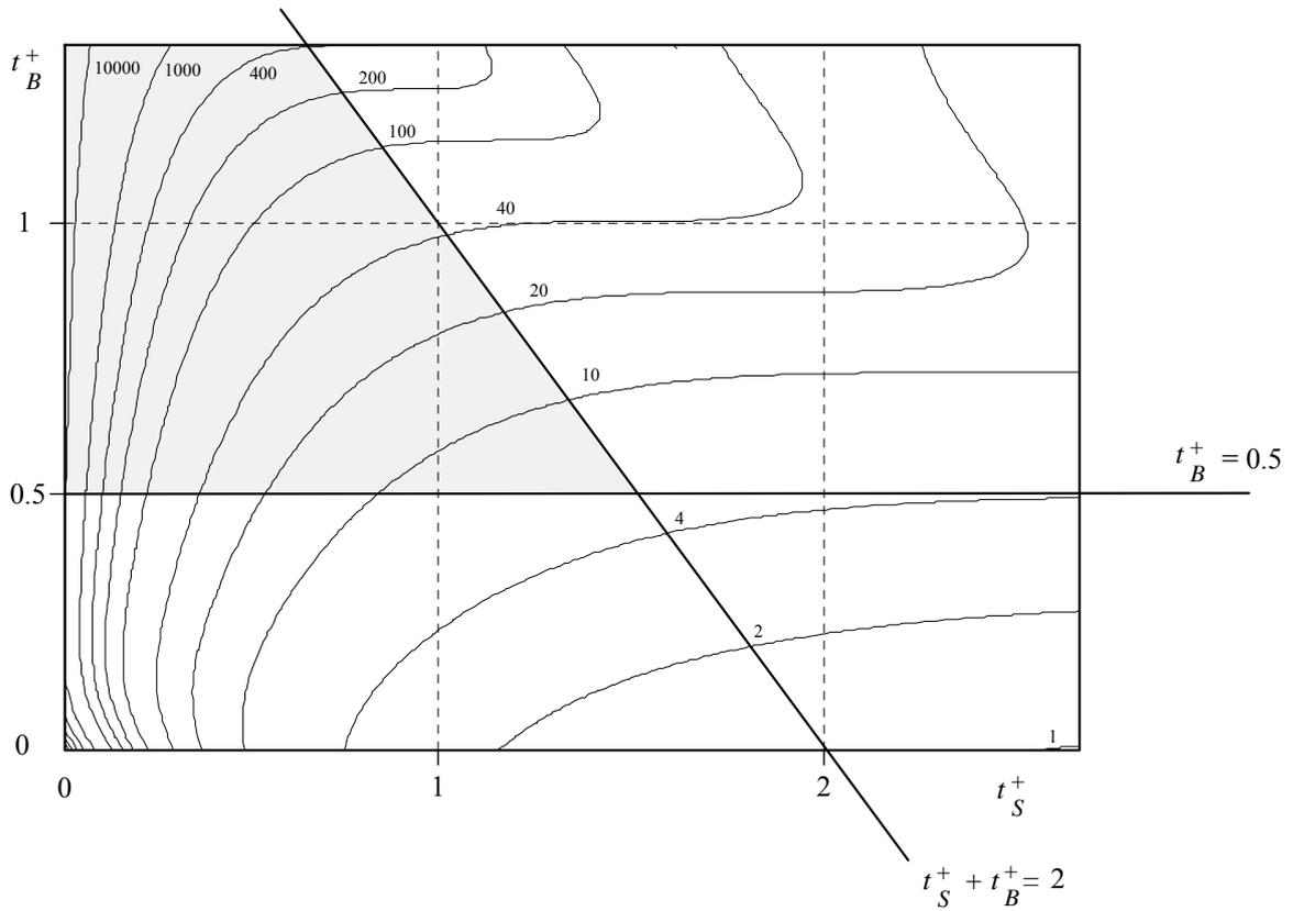
Fig 4 Contour plot of dimensionless coefficient  $A_a^+$  as a function of dimensionless times  $t_S^+$  and  $t_B^+$ .
