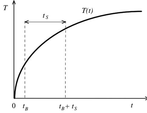
Fig 1 Temperature function and data window definition
