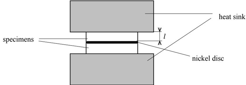
Fig 2 The setup of the experiment.
