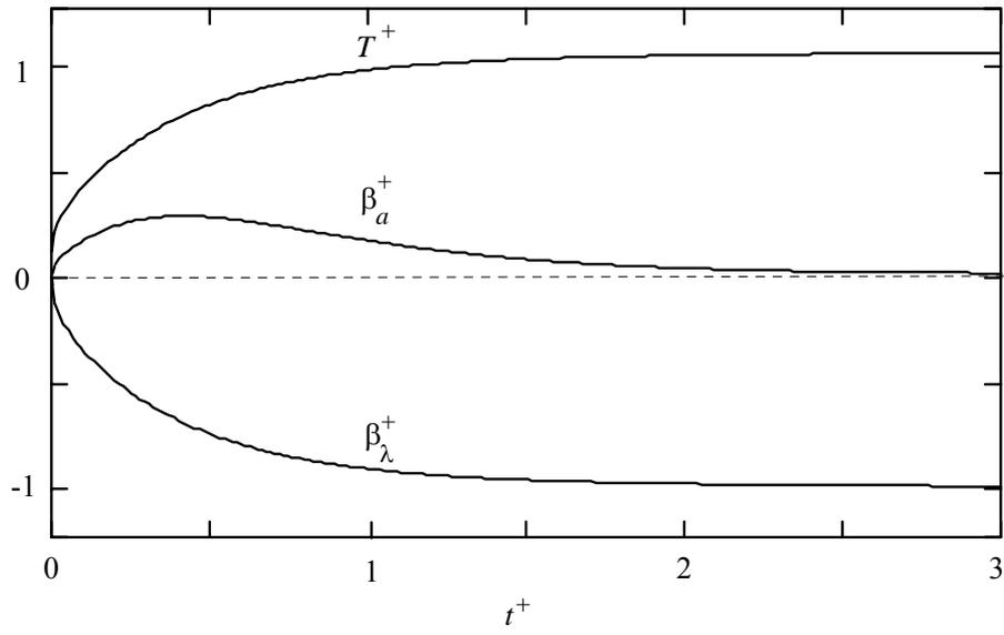
Fig 3 Dimensionless temperature function and dimensionless sensitivity coefficients  $\beta_a^+$  and  $\beta_\lambda^+$  vs. dimensionless time in EDPS method.
