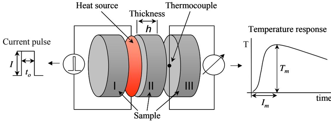
Fig 1 Experimental set up for Pulse transient method
