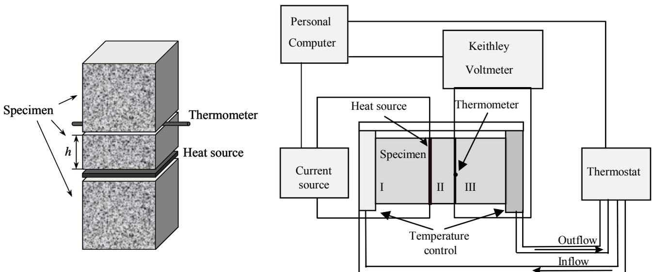
Fig 4 Specimen set-up (left) and basic scheme of instrument RTB 1.01(right)
