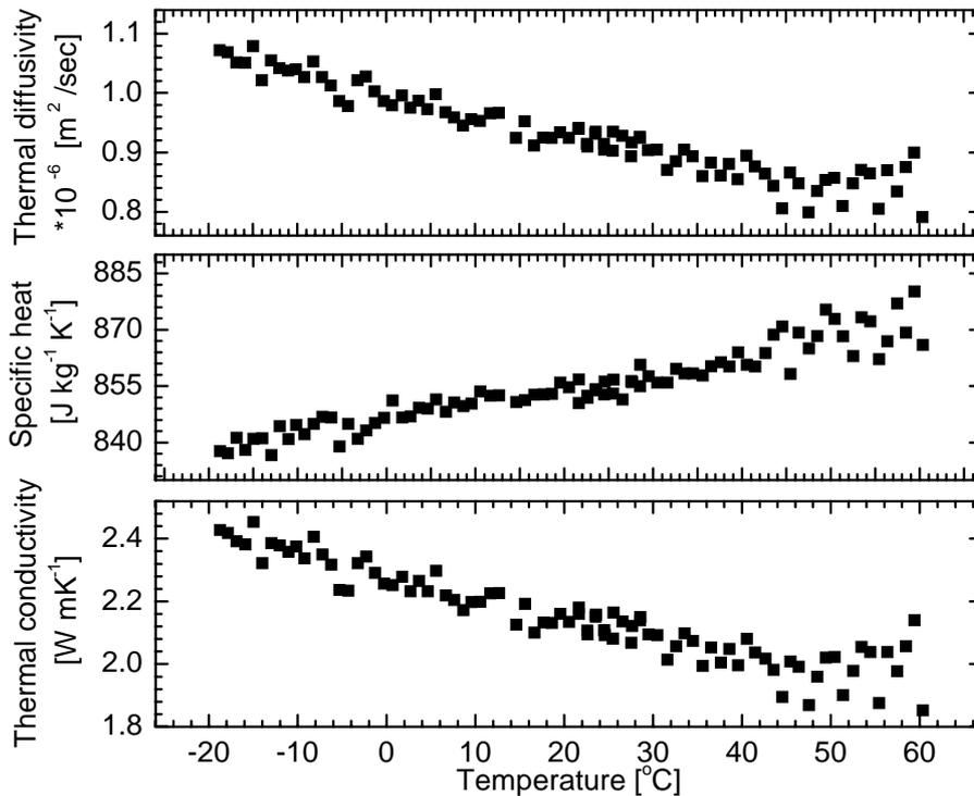
Fig 5 Thermophysical properties of dry homoblastic marble Gioia as a function of temperature
