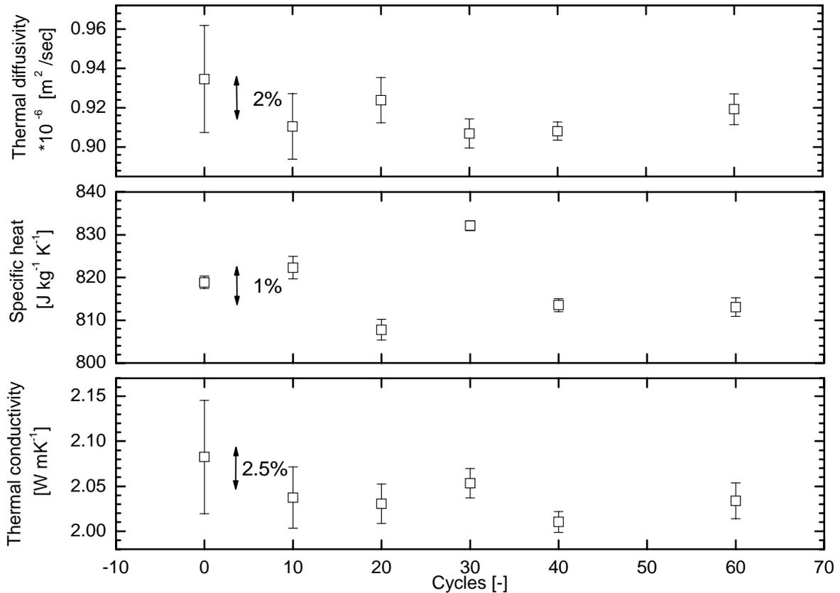
Fig 7 Artificial ageing of dry homoblastic marble Gioia (thermophysical properties in dependence on number of freeze/thaw cycles)
