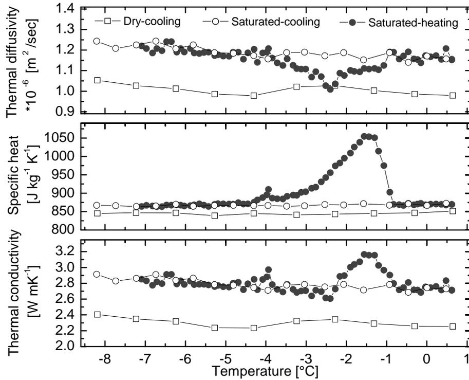
Fig 6 Thermophysical properties of dry and water-saturated homoblastic marble Gioia as a function of temperature during cooling and heating regime
